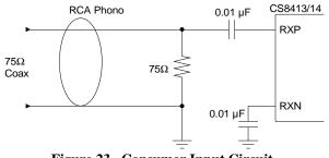
Figure 23. Consumer Input Circuit
