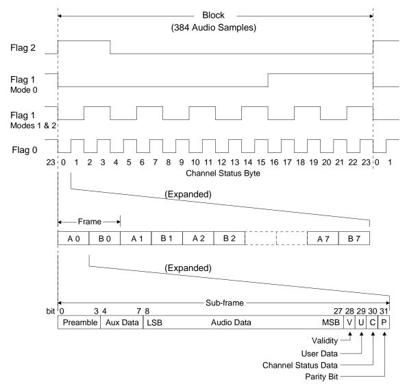
Figure 11. CS8413 Status Register Flag Timing
