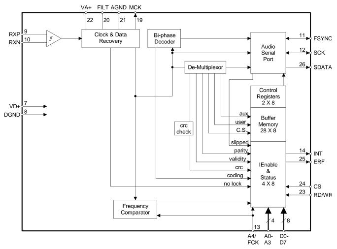
Figure 4. CS8413 Block Diagram
