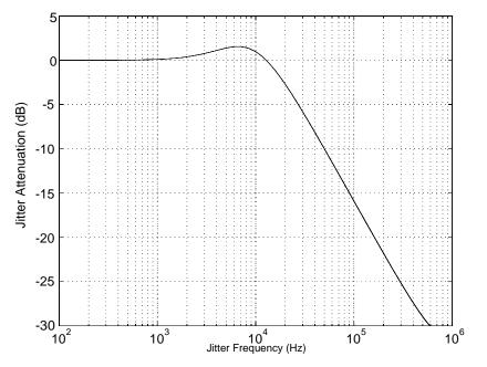
**Figure 3. Typical Jitter Attenuation Characteristics**
