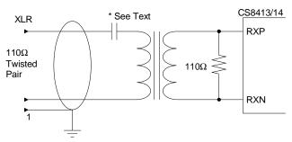
Figure 21. Professional Input Circuit
