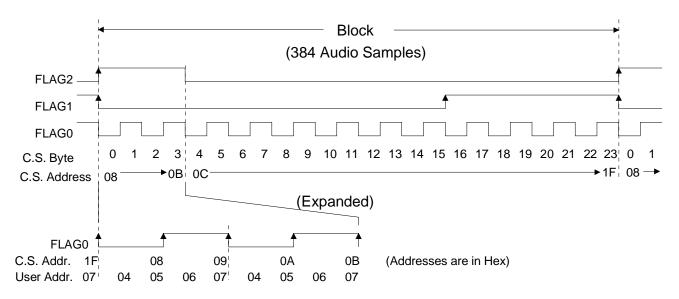
Figure 12. CS8413 Buffer Memory Write Sequence - MODE 0
