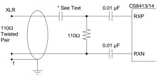
Figure 22. Transformerless Professional Circuit
