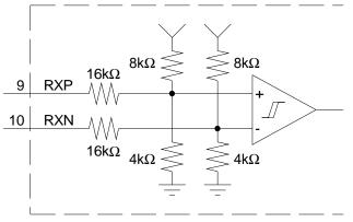
Figure 20. RS422 Receiver Internal Circuit
